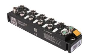
every TBEN-S module can be operated without additional gateways in each of the three Ethernet systems: PROFINET®, Modbus TCP ™or EtherNet/IP™. Additionally, thanks to TURCK's multiprotocol technology, the devices recognize the used protocol automatically by listening to the communication during the start-up phase. An integrated switch allows the use of the devices in line topology.
