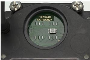
3. Triple click the button to put the master radio into binding mode.
